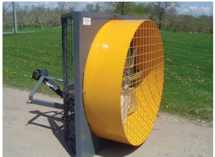
Figure 1. Example of PTO driven fan that can be used to increase barn ventilation.
