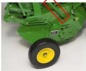
Semi-Pneumatic Gauge Wheels & Adjustable Float Springs
