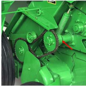
Chain Driven & Cutout-Clutch Protected
