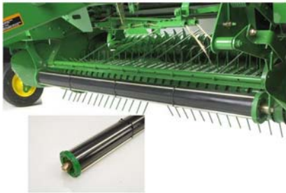
MegaWidePlus™ with Self-Adjusting Roller Baffle
